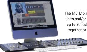
The MC Mix is designed to work with up to three additional MC Mix units and/or one MC Control to create a larger, integrated system with up to 36 faders. MC Mix and MC Control units can be elegantly clipped together or be situated anywhere on the network.
